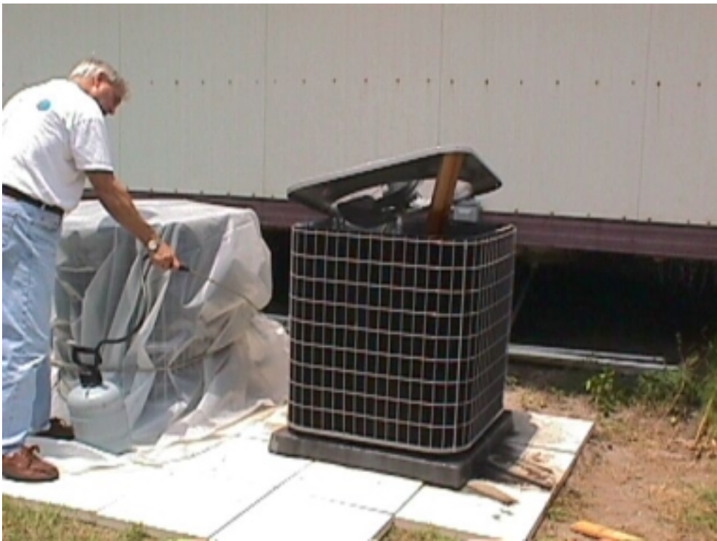
Figure 1. Installation of Two Carrier Condensers Side by Side for Test. Unit B1, the Adsil Unit Has Been Cleaned and Some of the Black Factory Coating Removed.
